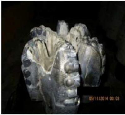
Figure 17—6" drill bit condition after pull out of hole, without the graphene enhanced lubricant. Bit was worn out with lots of solids sticking on it
