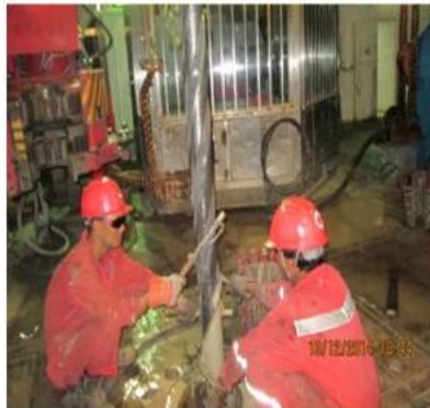
Figure 19—BHA condition during pull out of hole with graphene enhanced lubricant in the mud. BHA is cleared from any cuttings
